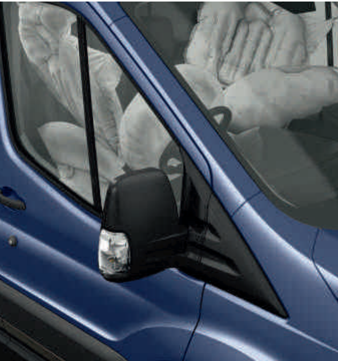
Side curtain airbags (1) Designed to help protect the driver and front passenger's heads from injury. (Option)
