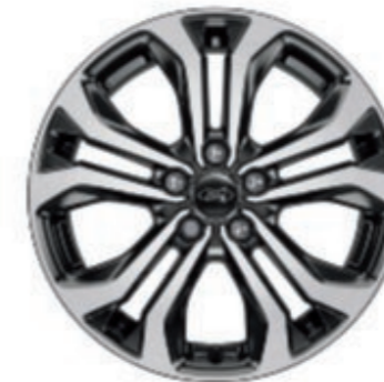
17" 5x2-spoke Black machined finish alloy wheel Standard on ST-Line (Fitted with 215/45 R17 tyres)
